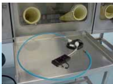
Gloves can be tested for leaks by use of a digital manometer or magnehelic gauge.
